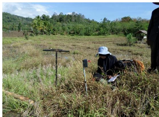
b. Examples of surface temperature measurement.
